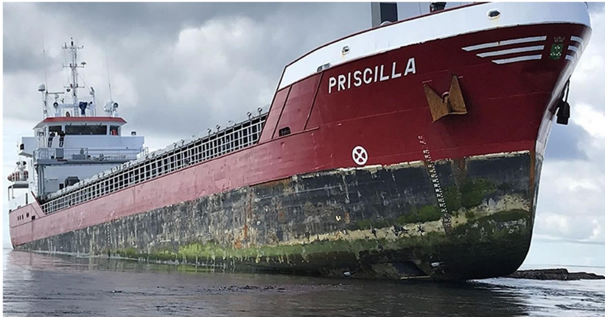
Figure 1 Grounded vessel Priscilla, after officer on watch was distracted by mobile device and was not keeping track on vessel's path taken from MAIB: Report on the investigation of the grounding of the general cargo vessel Priscilla on Pentland Skerries
